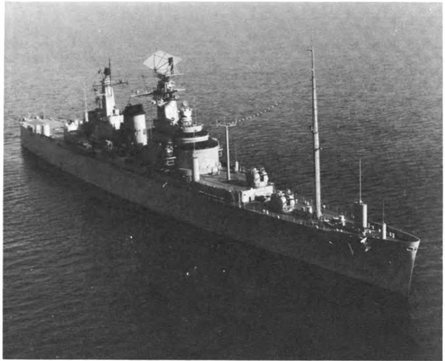
Figure 3. USS Northampton (ECLC-1), a cruiser commissioned in 1953. The antenna arrangements on the Northampton are as nearly ideal as developments to 1953 indicated would give the best communication efficiency.
