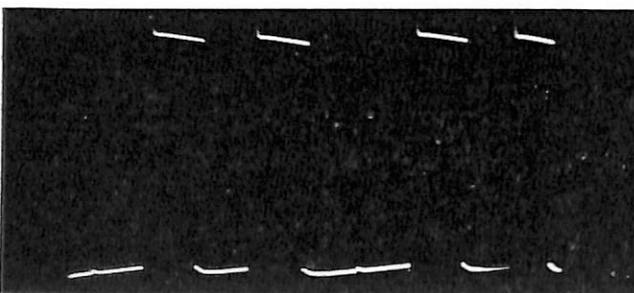
FIGURE 14c—Voltage wave on the collector of the second transistor of the second stage. Note the sharp pulse when this unit is stepped back.
