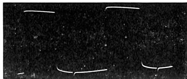
FIGURE 14d—Voltage wave on the collector of the third stage. Note the sharp pulse when this unit is stepped back.
