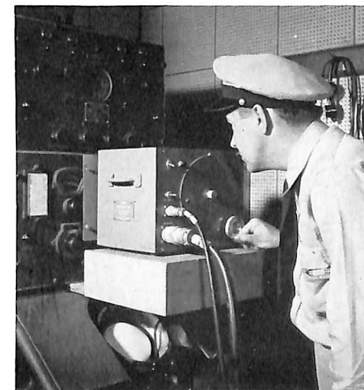
Radio follower unit connected to dial of DAK-2 receiver.
