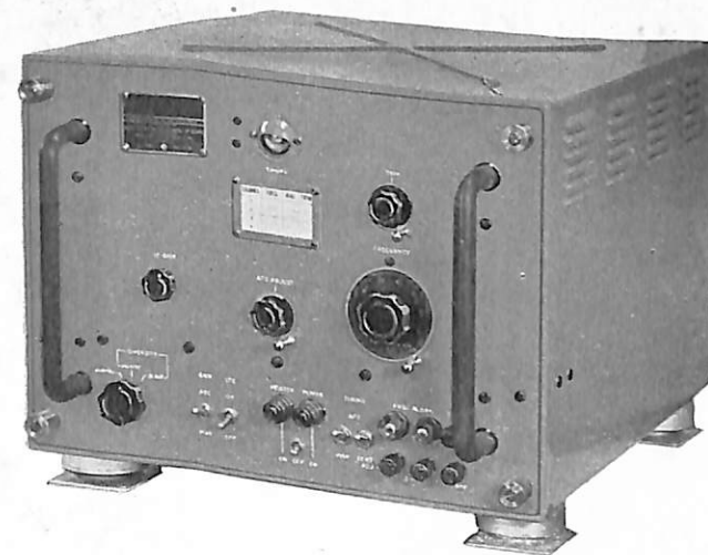
FIGURE 10—Radio Receiver R-360/SRR-4, one of two utilized in the Radio Receiving Equipment AN/SRR-4.
