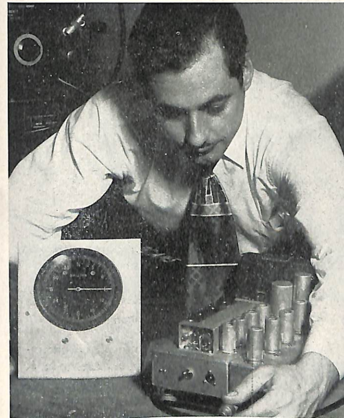
Alignment of experimental rotating pulse beacon transmitting equipment.
