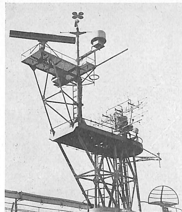
FIGURE 9—IFF Directional Antenna AN/UPA-11 mounted on upper left platform on a light aircraft carrier.
