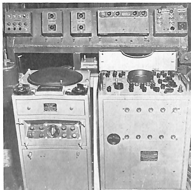
FIGURE 14—Interconnection Assembly UPA-9 Indicator with associated VJ repeater located in CIC of a light aircraft carrier. UPA-9 indicator is on right. Control boxes above are units of the Mark V IFF System.
