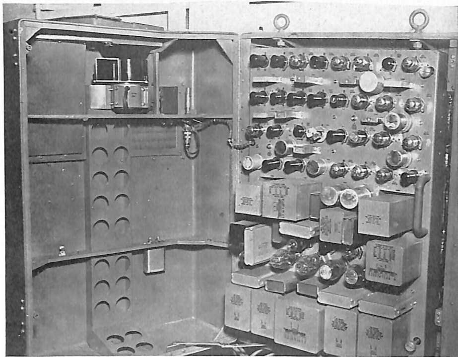
FIGURE 13—Interconnection Assembly UPA-9 Synchronizer with front panel open to show the mounting arrangement of components on inner panel.
