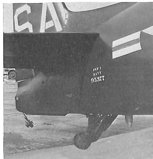
FIGURE 10—Airborne omni-directional antenna AS-133 mounted on underside of fuselage of Naval aircraft.
