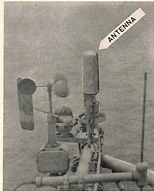
FIGURE 11—Surface transponder omni-directional antenna AS-177 located on forward port yardarm of a heavy cruiser.
