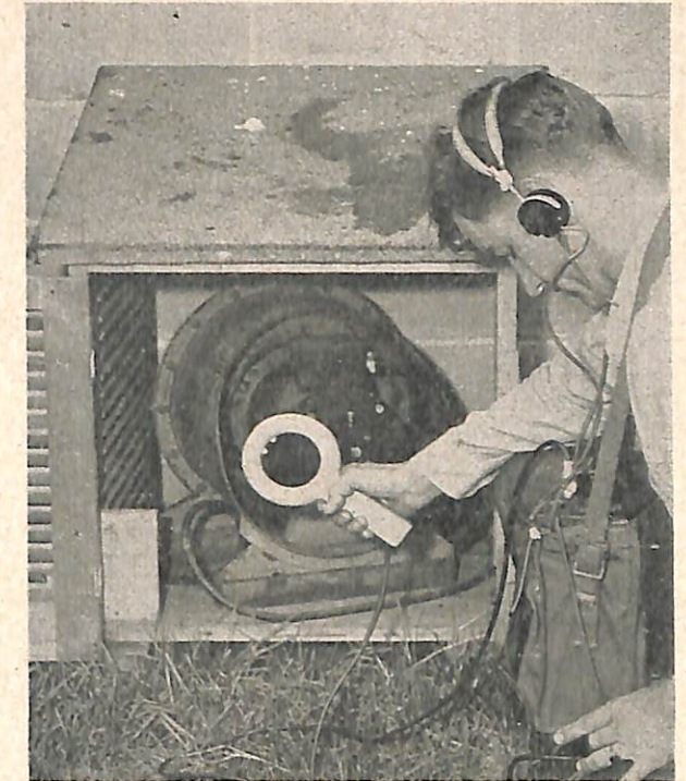
Using the Eltron radio noise locator to detect radio interference created by the turbo-jet motor of a Link Trainer.
