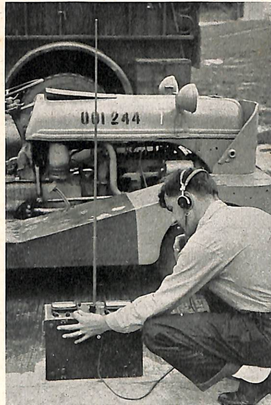
Using the Model OF-2 to measure the radiated ignition interference of an aircraft tow tractor.
