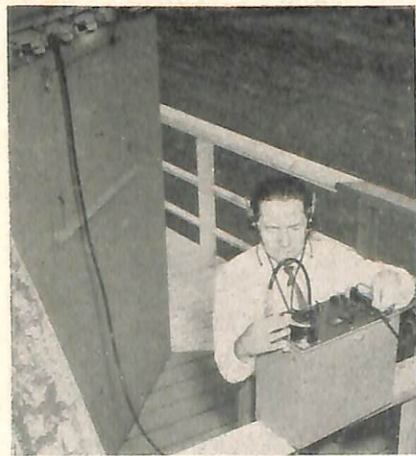
Model AN/PRM-1 directly connected to the antenna input of a control tower radio receiver.
