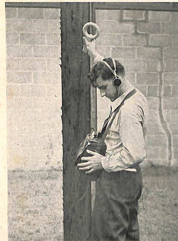
Detecting power line radiated interference with the Eltron radio noise locator.
