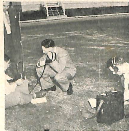
Using the Model AN/PRM-1 to measure radiated radio interference intensities, with a loop and rod antenna. Note the Ferris Model 32A on the right being used for comparative readings.
