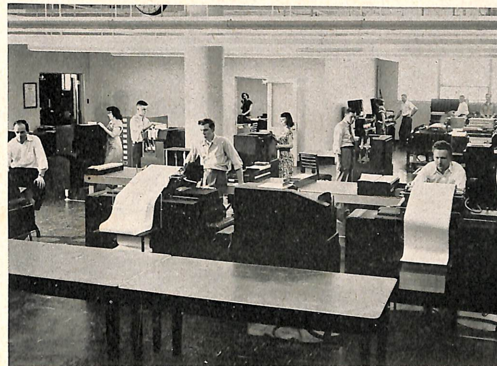
ELECTRIC ACCOUNTING MACHINES interpret, sort, merge and list information from EAM cards.
