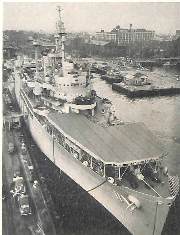
Forward view of the U.S.S. NORTON SOUND, showing the miniature flight deck for the landing of helicopters and launching of balloons.
