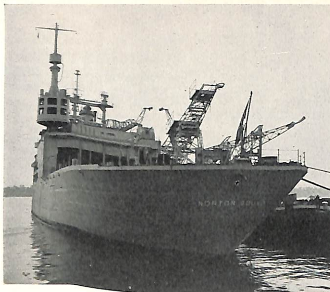
Stern view of the U.S.S. NORTON SOUND, showing the ADJUSTABLE ROCKET LAUNCHING RACKS capable of launching V-2 type rockets as well as the smaller "Aerobees."
