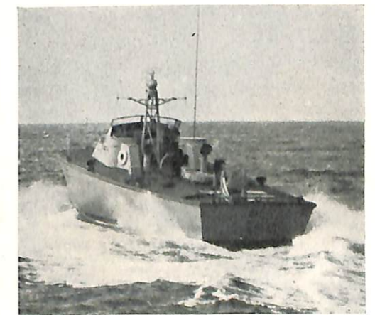
NOBODY HOME. At left, Lt. R. F. Murray aboard RCT-15, controlling RCT-14 at the right. At right, RCT-14 under radio control, leaving RCT-15.
