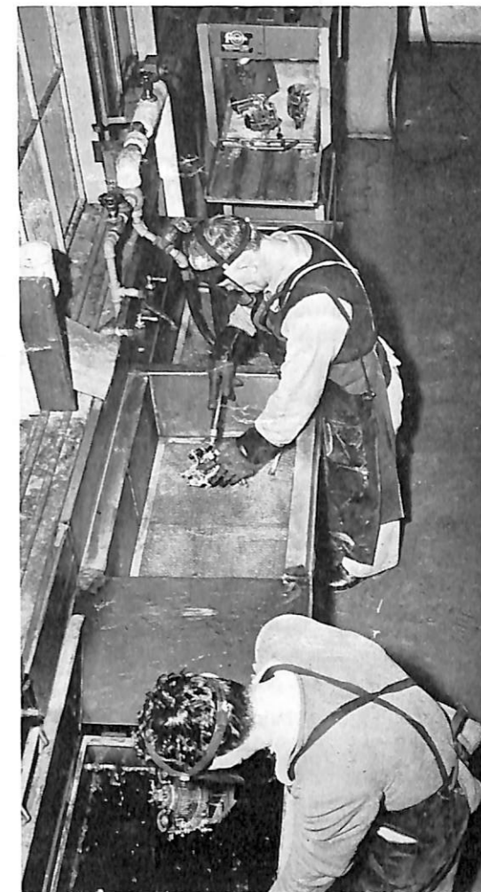
DISASSEMBLED TELETYPE UNITS being sprayed with cleaning solvent.
