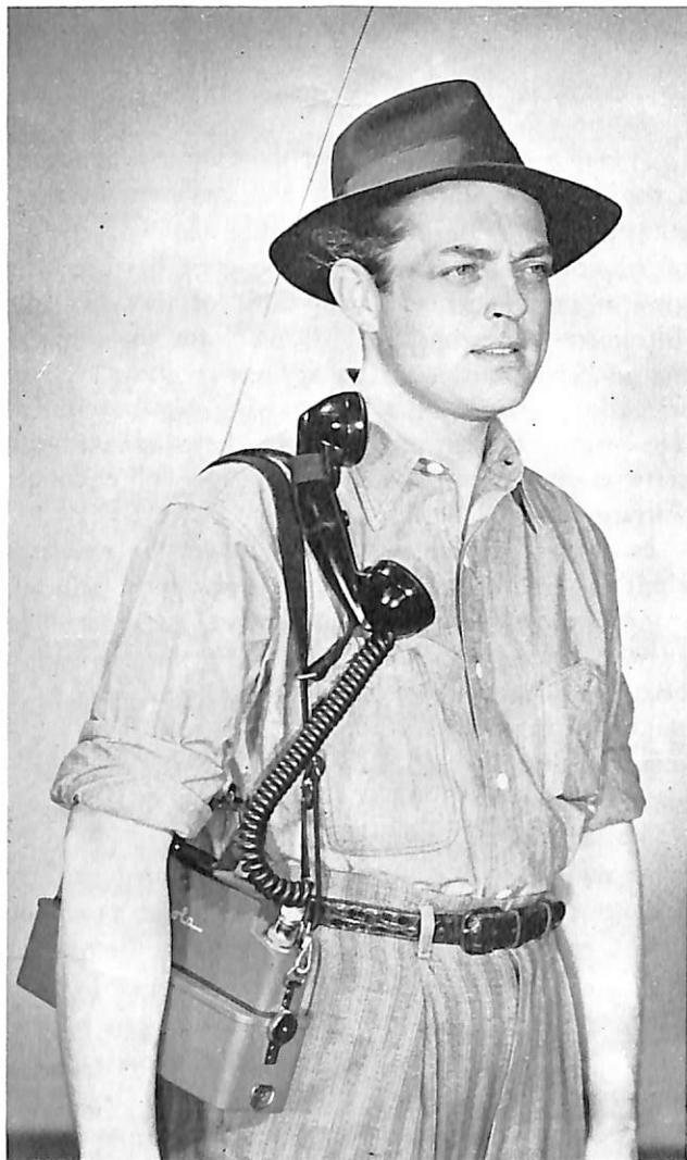
One of the many operating positions possible with the Motorola FM HANDIE-TALKIE UNIT.
