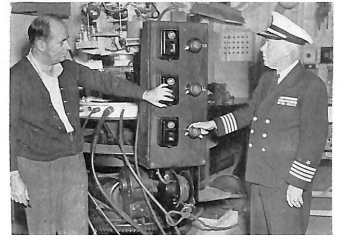
CAPT. BEATTIE is shown the test stand for checking SP stable elements by MR. FRANK THEMER, Electronics Engineer. Radar stable elements constitute a large part of the work load of this shop.
