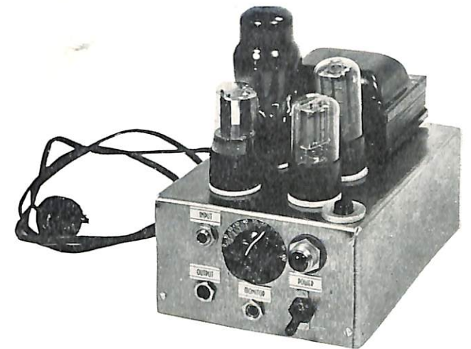
FIGURE 2—"On-off" radio-teletype adapter operates teleprinters from standard Navy receivers.
