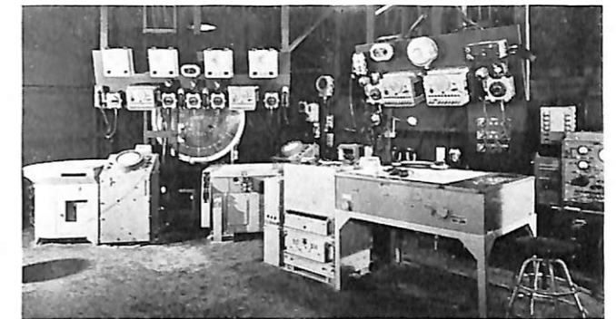
CV C.I.C. showing air and surface fiddle boards, D.R.T., radar repeaters, horizontal and vertical air plots.
