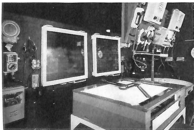
DD C.I.C. showing observer's platform, D.R.A., status boards, fiddle boards, D.R.T., and radio receivers.
