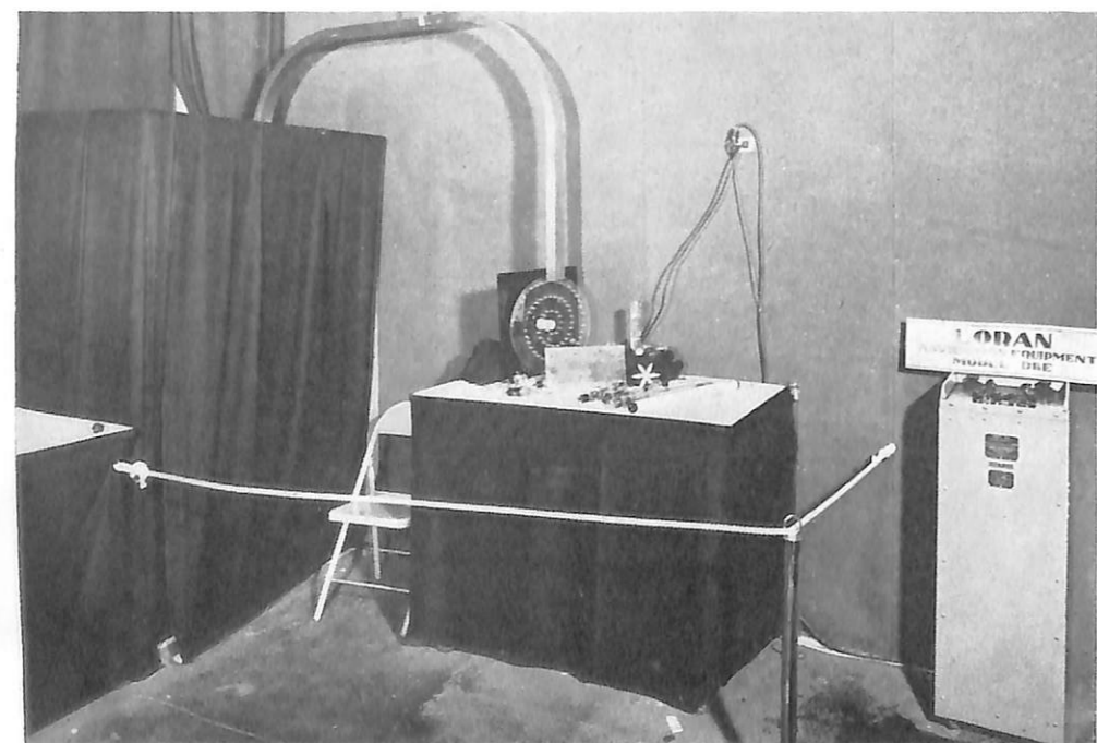
Radio frequency exhibit. Energy from the open end of the model SV radar transmitter lighted argon lamps on display racks.
