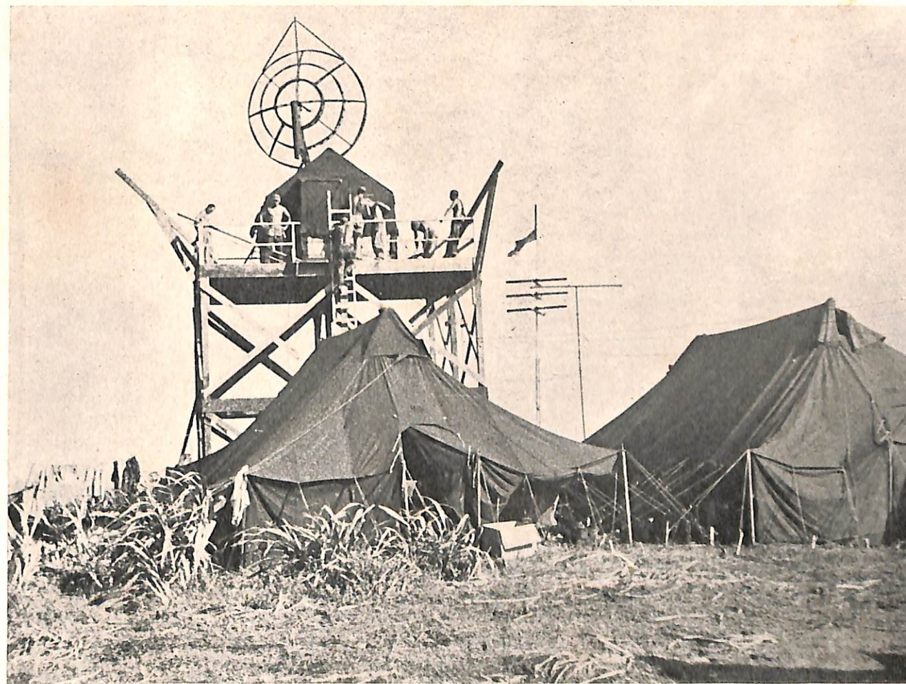
FIGURE 78—AN/TPS-3 set placed on tower to clear surrounding obstacles.
