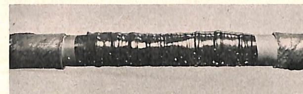
FIGURE 5—Cable ready for molding of the vinylite jacket. Note the vinylite tape wound in layers over the copper braid.
