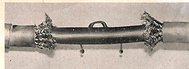
FIGURE 3—Polyethylene dielectric after the mold is removed.
