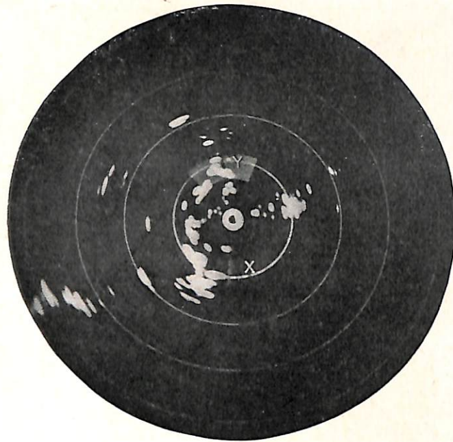
PPI screen showing target presentation, range marks, intensified ribbon marker X, and segment selected for enlargement Y.
