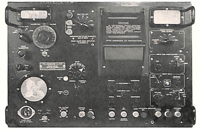
Front panel of the TS-239/UP Oscilloscope. The CRO tube is not visible until the light shield, upper right, is lifted. The screens at three of the corners are for ventilation.
